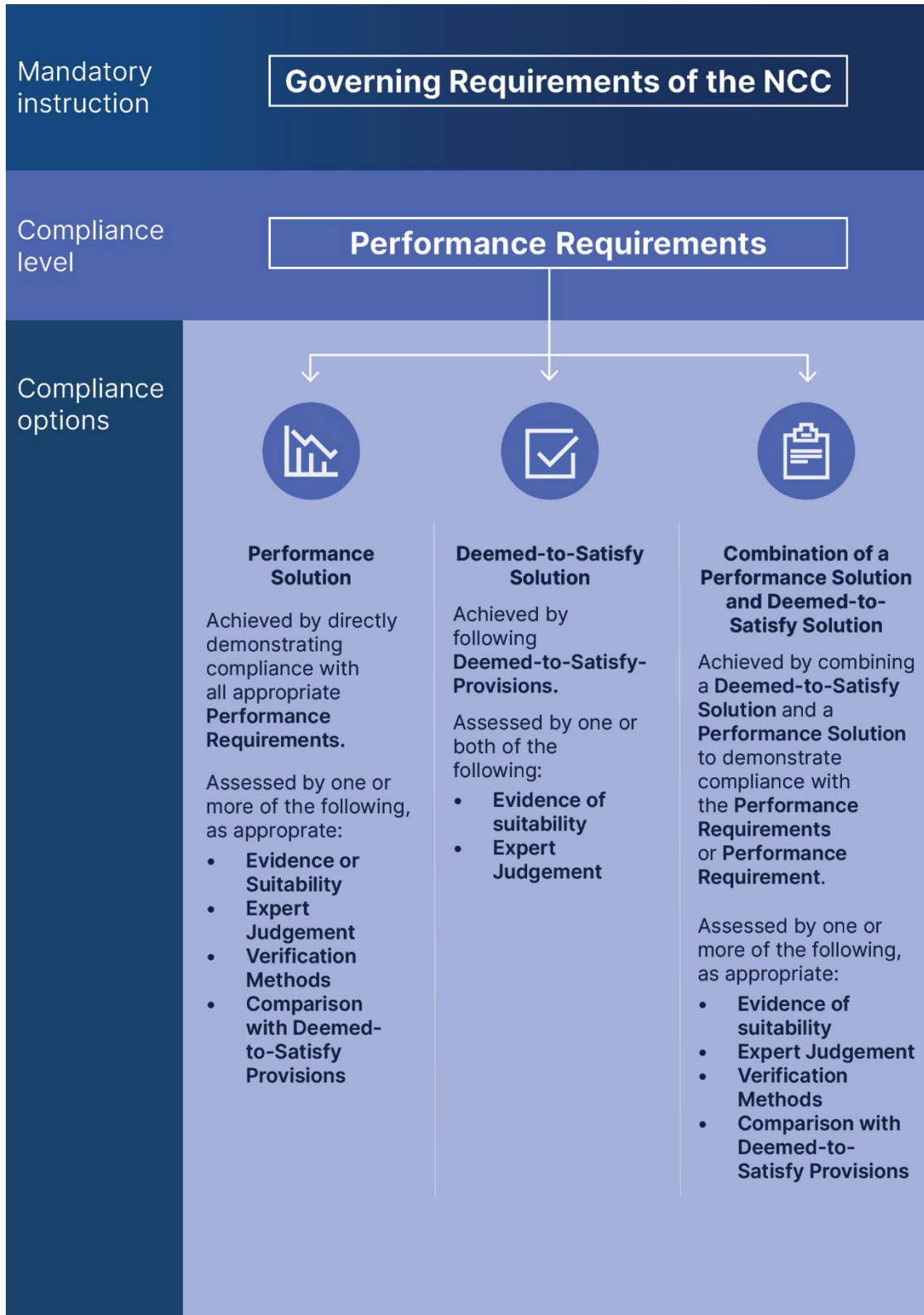
Figure B.1 Demonstrating compliance with the NCC
