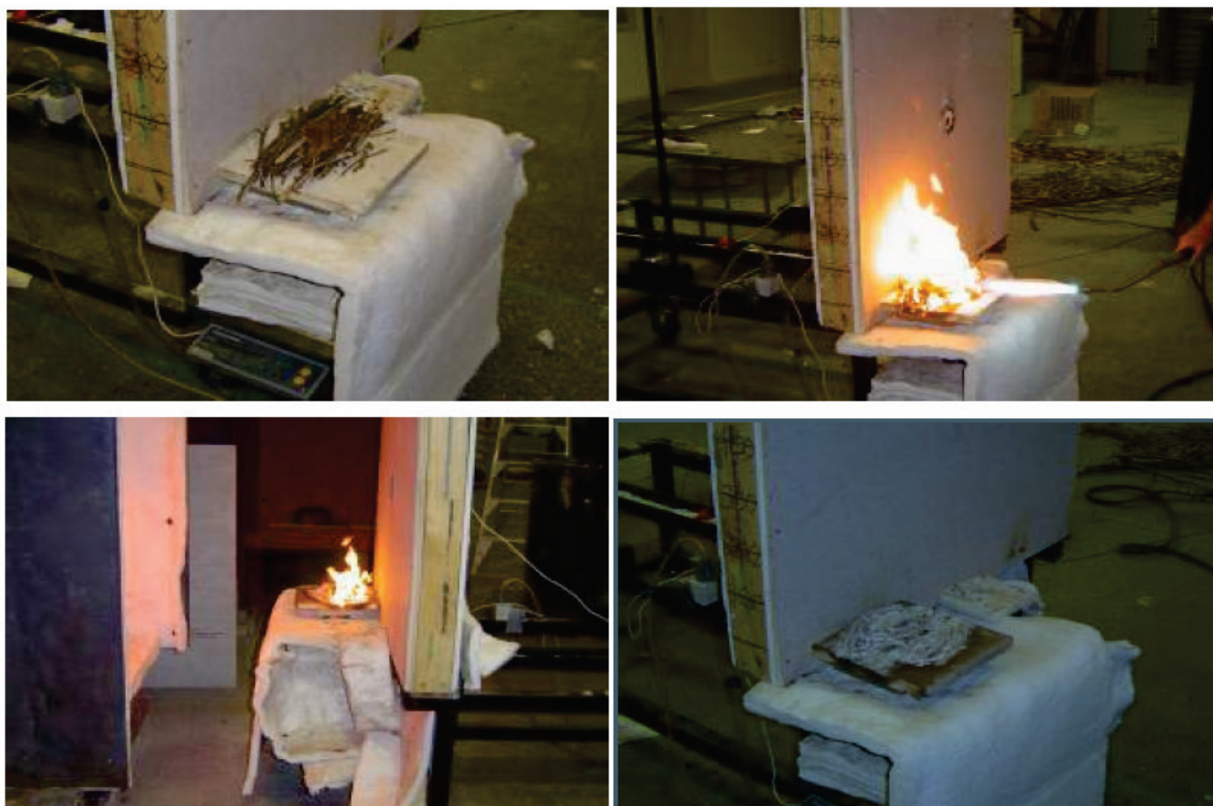
Figure 5.10 Determination of mass burning rate for debris when exposed to radiant heat (England et al. 2008)
